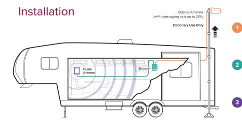
**Receives signal:** The powerful antenna reaches out to access existing outside signal from nearby cell towers and delivers it to the booster.
