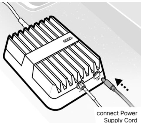
For CLA power option; plug into vehicle's 12V DC Power Supply
